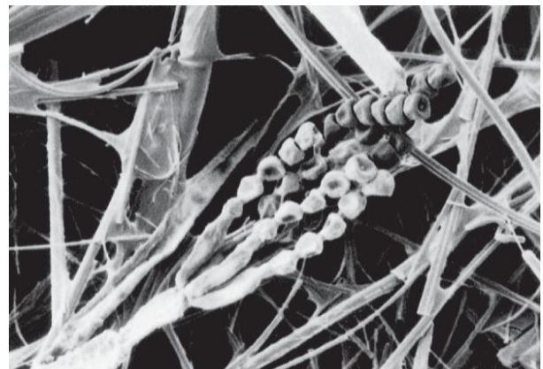
Fungus Build-Up on Conventional Filter
